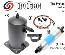
The Protec Anti-Surge kit eliminates fuel surge and reduces the risk of cavitation in the primary pump. The bypass valve controls the pressure inside the pot, any excess fuel is then returned back to the main fuel tank.
